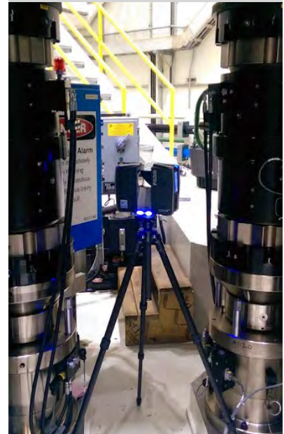
Data Capture with a Faro Focus3D
